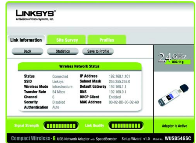
Figure 5-3: Link Information - Wireless Network Status
